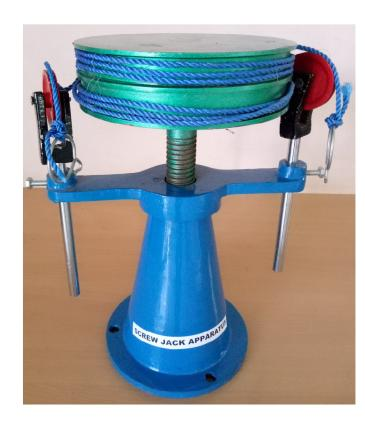
Apparatus consists of a metallic machined screw with a pitch of 5mm carrying a double flanged turned table of about 20cm dia. Screw jack is fitted on a heavy C.I. base and is supplied complete with 2 adjustable pulleys, cord and hooks.
